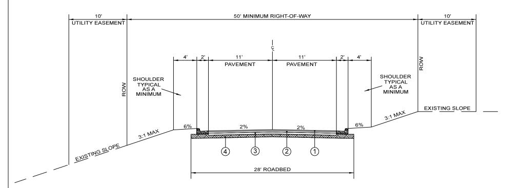
WEARING SURFACE: 1" Required Improved Bituminous Concrete Wearing Surface Layer, Type 424, 110 Pounds Per Square Yard.
