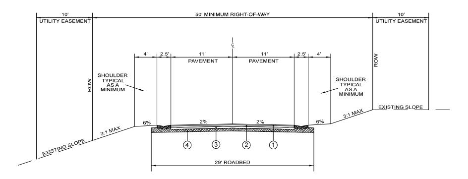
WEARING SURFACE: 1" Required Improved Bituminous Concrete Wearing Surface Layer, Type 424, 110 Pounds Per Square Yard.
